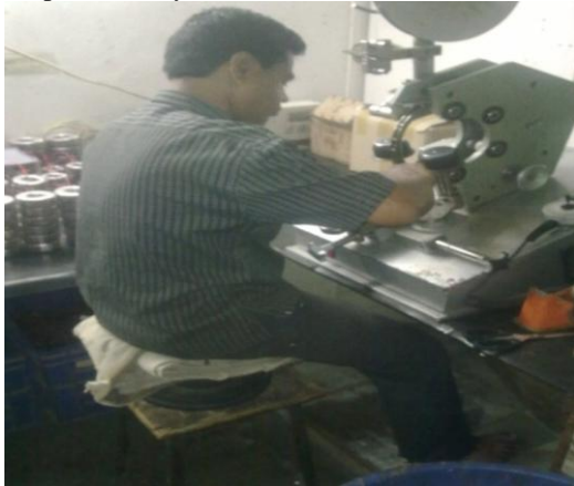
Fig.1 A typical working posture adapted in order to perform Transformer winding operation.
